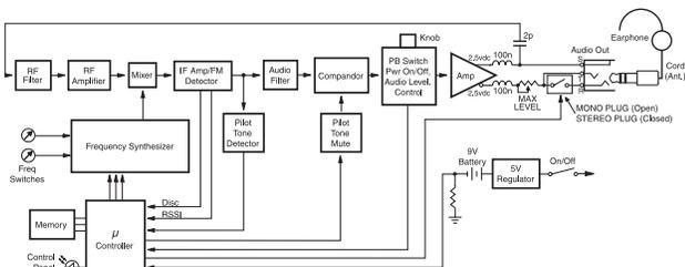
Figure 4 - R1a Block Diagram
