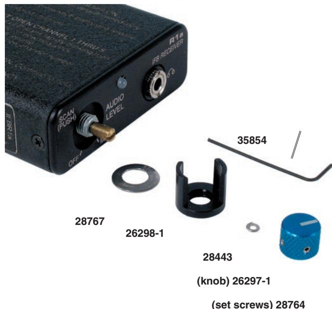
**Note:** If you wish to change the frequency or mode and the knob is unable to be depressed, check to see if this procedure has already been done. You can temporarily enable the functions if you loosen the set screw, pull the knob out a small amount, tighten the set screw, and depress the knob. Then, reverse the procedure to disable the knob again. However, if you wish to permanently enable the knob, replace the spacer washer between the knob and the shaft.
