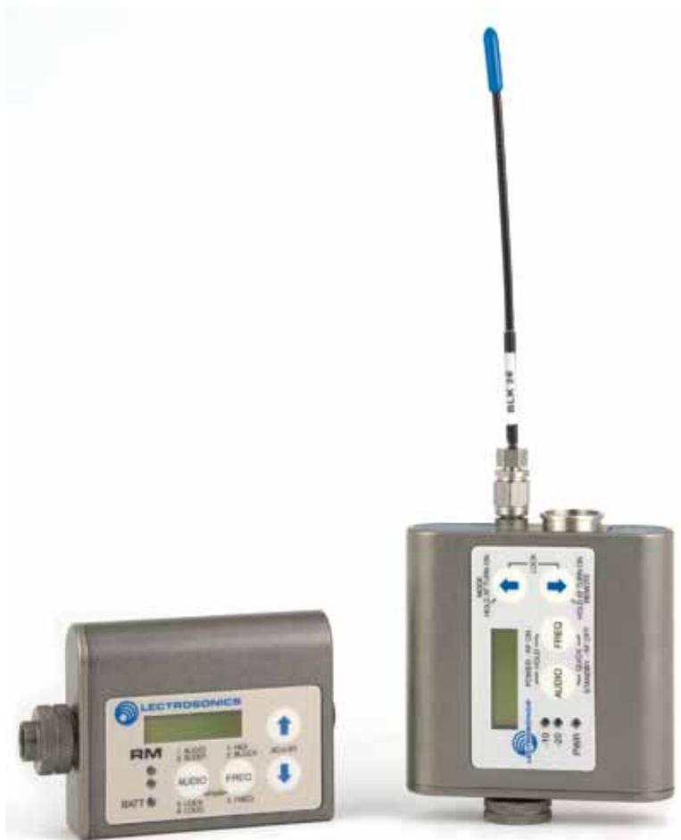
A water resistant control panel with LCD, membrane switches and multi-color LEDs make input gain adjustments, frequency and compatibility mode selection quick and accurate. The battery compartment accepts lithium or rechargeable AA batteries.
